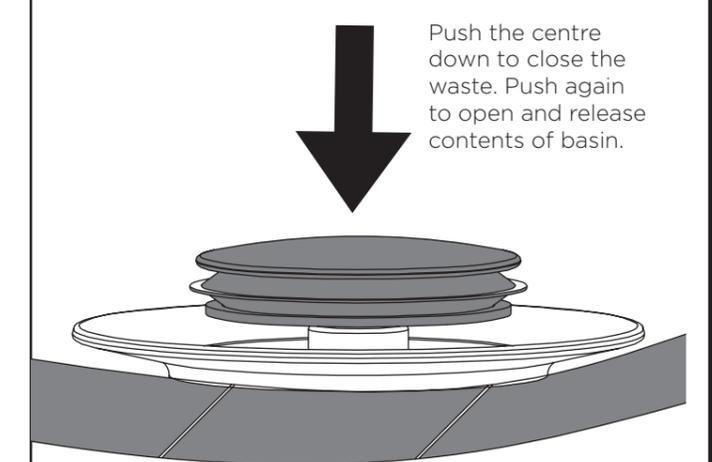
Push the centre down to close the waste. Push again to open and release contents of basin.
