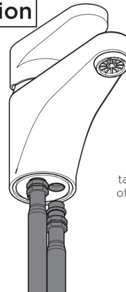
Screw the copper tails into the bottom of the mixer body by **hand only**. (DO NOT OVERTIGHTEN)
