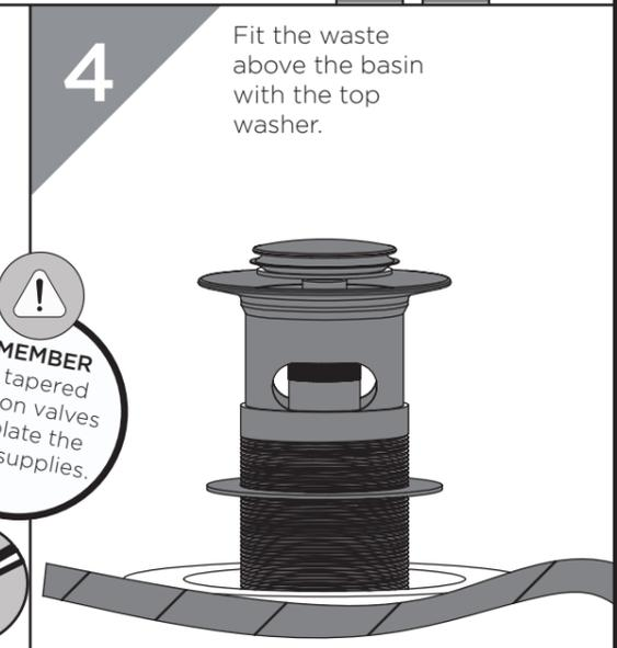
Fit the waste above the basin with the top washer.
