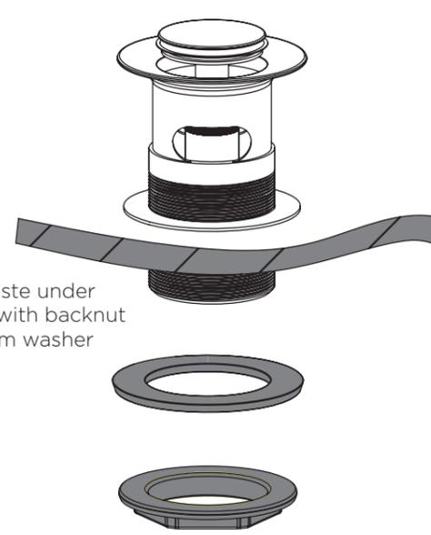
Secure waste under the basin with backnut and bottom washer
