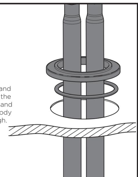
Place the plinth and the washer over the hole in the basin and feed the mixer body and tails through.
