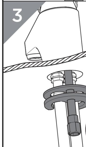
Secure to basin using fixing kit, connect the hot and cold water supplies to the tails.
