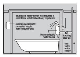
Plan your own installation carefully. Check on the nearest and most readily accessible rising mains water supply, this may be beneath the bath or in the loft, where it feeds the cold water storage tank. Use only the cold rising water main supply.
