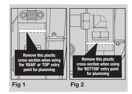
The back plate is fitted with removable inserts for **Top** (falling) and **Bottom** (rising) inlet mains water pipework to the shower unit.
