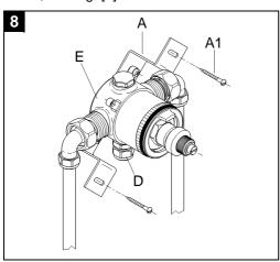
4. Connect mixed water supply to the outlet nipple (D).
