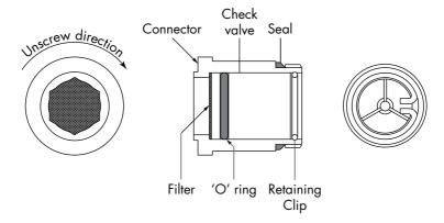
Using a 12mm A/F hexagon wrench unscrew both connectors and the body.
