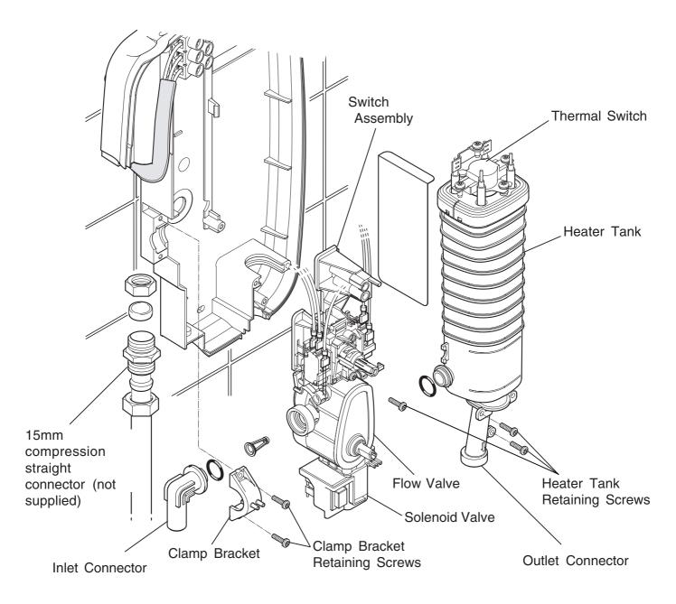
Heater Tank - Removal and Installation
