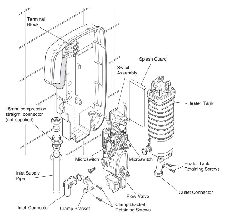
Flow Valve and Switch Assembly - Removal and Installation
