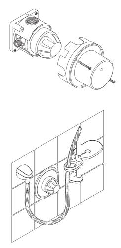
Mark the wall surface for an opening measuring approximately 245 mm x 125 mm.
