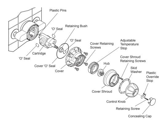
Push the cartridge fully into the shower control body. Make sure that the two plastic pins locate in the brass body recess.
