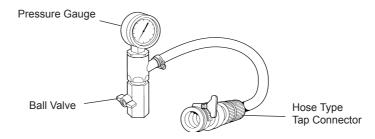
**Pressure Testing Device**
