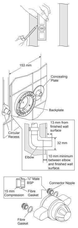
**2.7** Fit the Compression Nuts and Olives onto the pipework.
