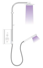
Switch water flow from overhead to handset 2-3 times to test operation.
