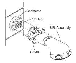
**17.** Fix the upper shroud to the BIR assembly using the four self-tapping screws provided.
