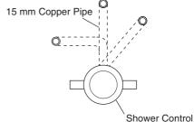
The end of the 15 mm copper pipework must protrude through the finished wall surface by 23–25 mm.
