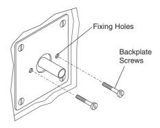
**13.** Fix the backplate to the wall using the two backplate screws.
