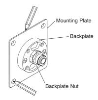
Fit the mounting plate to the wall with the four mounting plate screws supplied. The two threaded holes must be horizontal.
