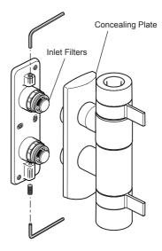
**12.** Push the concealing plate onto the backplate, secure with the M4 x 12 mm grubscrew.
