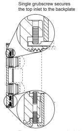
Two grubscrews secure both the bottom inlet and the concealing plate to the backplate
