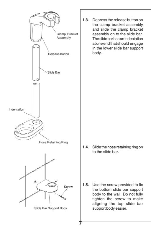
**1.6.** Push the slide bar, complete with the previously assembled components, into the recess in the bottom slide bar support body. Rotate the slide bar until the **indentation** engages in the slide bar support body.
