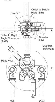
2. Remove the plasterboard and or brickwork to a minimum depth of 55 mm depth so that the outlet of the Rada V12 mixer aligns with the diverter inlet.
