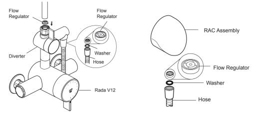
**Note!** If the diverter is installed with the Rada VR range of showerheads, a 9 l/min flow regulator is factory fitted in the showerhead. If a 6 l/min flow regulator is required, the 9 l/min flow regulator should be removed from the showerhead.
