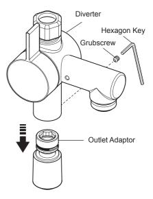
Install the outlet adaptor and the 'O' seal (supplied) onto the V12 mixer outlet and fully tighten using the 'O' key or 12 mm hexagon key.
