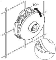
**Note!** The **number 1** on the concealing plate should be positioned at the top.
