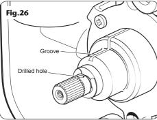
onto the splined spindle. When fitting the temperature control, the pointer must relate to the '5' on the temperature scale when the cover is fitted **(fig.25)**. Refit the retaining screw and push fit the cover trim back into place.
