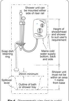
Fig.6 Diagrammatic view (not to scale)
