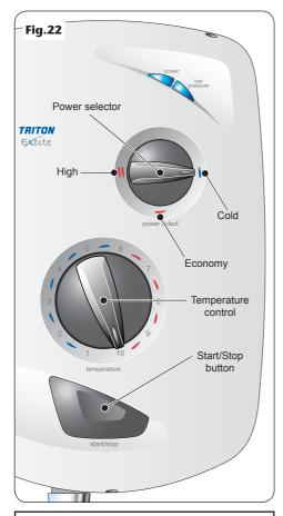
**Note:** In normal use, it is in order to leave the water supply permanently on to the shower unit, but as with most electrical appliances, **the unit must be switched off at the isolating switch when not in use.**
