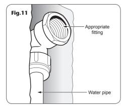
Remove the valve and drill the holes. Route the pipework to the valve position.
