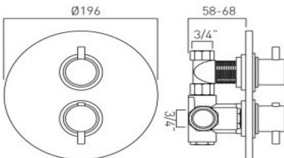
**description:** concealed 2 handle thermostatic shower valve wall mounted with round backplate thermostatic cartridge V-001C-PLA flow cartridge CEL-002A/B-3/4 2 x 3/4" female inlets 1 x 3/4" female outlet includes fittings for 1/2" and 3/4" pipework min-max wall mount 58-68mm (standard) optimum installation depth 63mm (standard) min-max wall mount 68-96mm (extension option) optimum installation depth 82mm (extension option)
